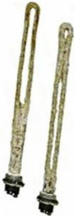
Typical electric water heaters utilize **metal heating elements** to heat water in a large storage tank. The metal elements attract minerals in the water and develop a corrosive scale that reduces the efficiency of the water heater. If you don't spend hundreds of dollars each year to flush and descale the water heater, it will eventually fail. In addition, electricity is also used during the day and night to maintain the temperature of the water in the tank whether you are using it or not.
