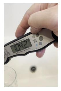
**Test 2:** The temperature on the SIO 18 Pro was increased to 120 degrees and the test was run again. This time the shower ran for 60 minutes (90 Gallons) and the gas heater never came on. Also, the gas heater did not go into recovery mode to reheat any water.
