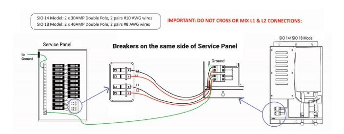
SIO 14 Model: 2 x 30AMP Double Pole, 2 pairs #10 AWG wires SIO 18 Model: 2 x 40AMP Double Pole, 2 pairs #8 AWG wires
