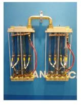
This heating element was removed for inspection from an early prototype unit installed in 2010 during the R&D period. This array ran 9 hours/day, 365 days/year for over 7 ½ years in a nail salon with no scale, no maintenance and no loss of efficiency. The only minor issue was a slight discoloration on one tube from insulation.
